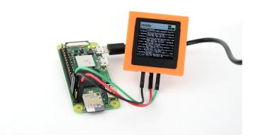
In addition to working as a USB powered peripheral, TermDriver can run in standalone mode with no USB connection. In this mode 3.3 V power is supplied by the target circuit. Connect GND, 3.3V and RX to the target circuit.
