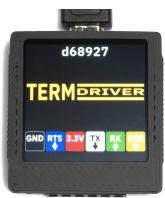
TermDriver2 has 6 output pins, on a standard 2.54 mm (0.1") female header.
